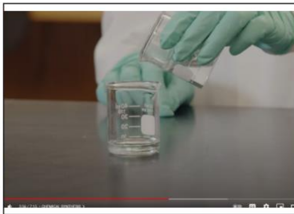
Never return unused reagents to the bottle close-up shot of the chemical being poured
