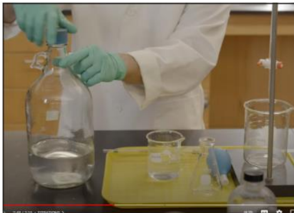
Never return unused reagents to the bottle Student pour from the stock bottle to the beaker
